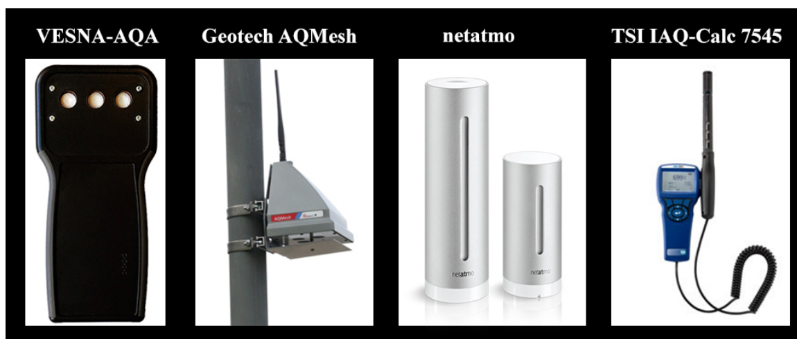
Figure 5: Sensor units used at the case study school.
