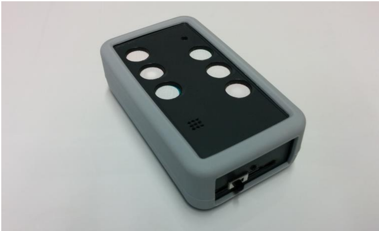
Figure 14-1 The VESNA v2.0 Personal Air Quality (PAQ) Sensor Pack
