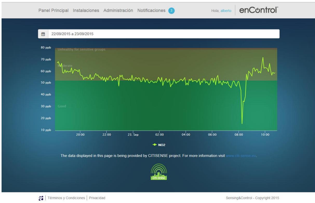
Figure 10-6: Nitrogen Dioxide (NO 2 ) raw data aggregated (avg) on 5 minute interval with AQI
