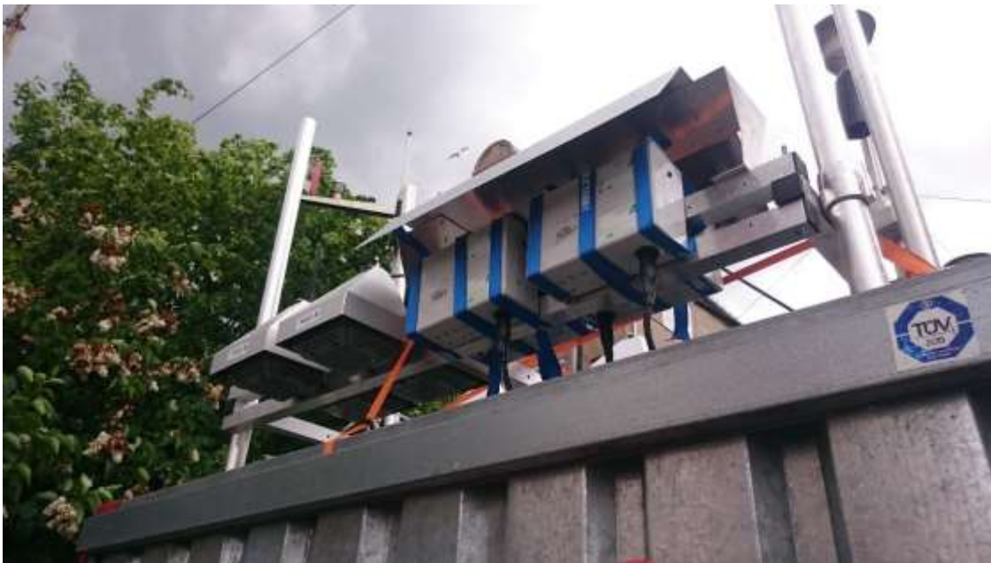
Figure.28 Picture of the measurement set-up of 4 Atmospheric Sensor platforms co-located together with the air quality station of Kirkeveien.
