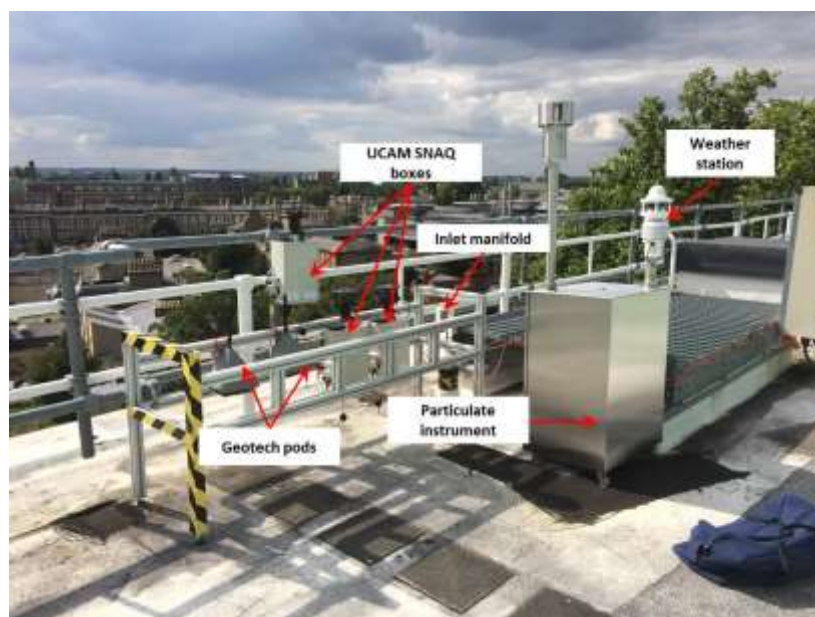
Figure 1. Layout of gas measurement (a) and actual setup of instrument suite (b).
