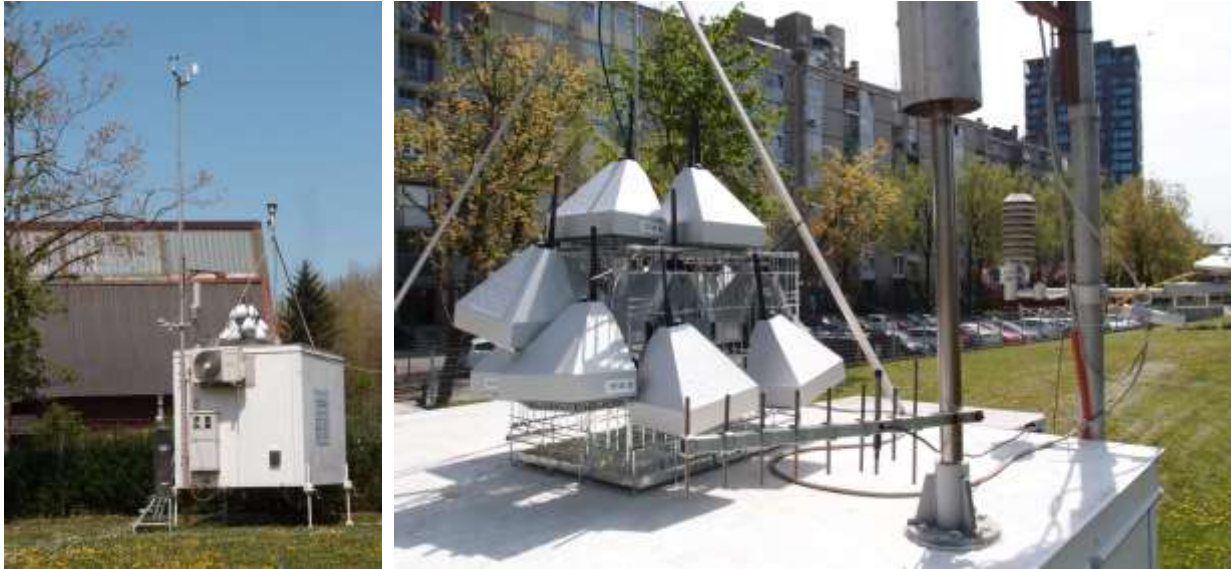
Figure F1: Pictures of the measurement set-up of 17 AQMesh pods co-located together with the reference air quality station in Ljubljana.
