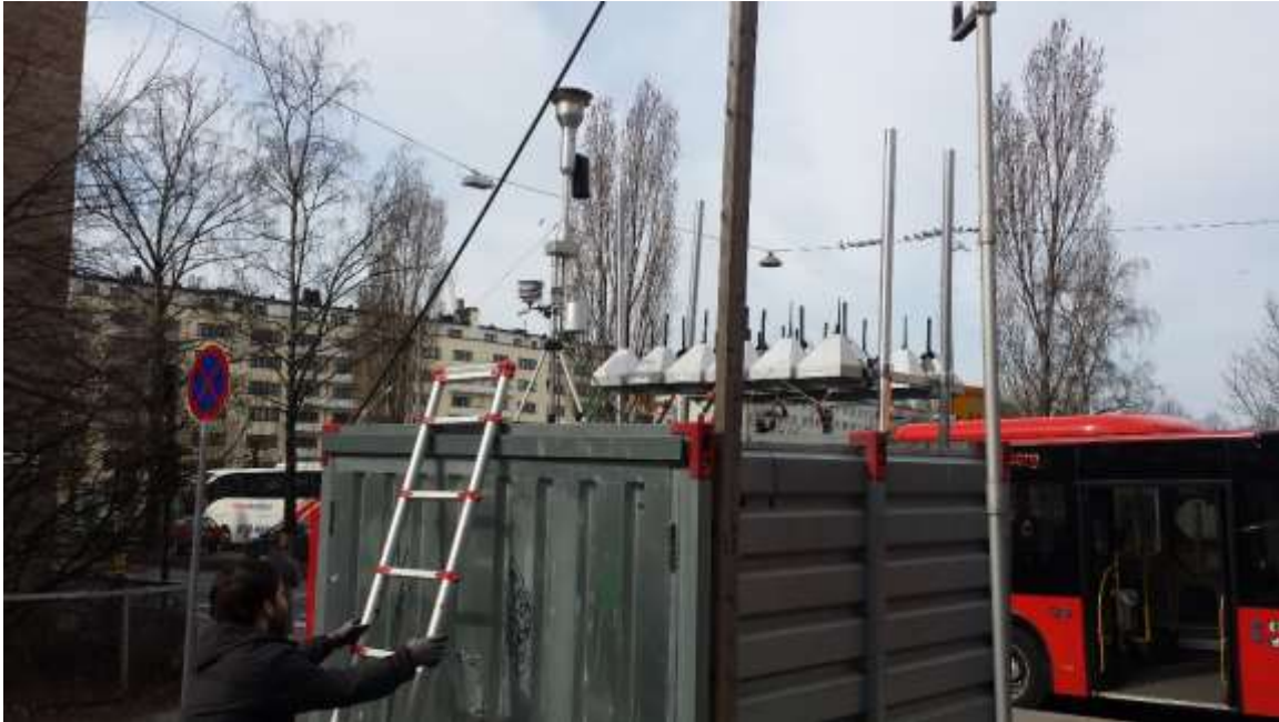
Figure.27 Picture of the measurement set-up of the 24 Geotech/AQMesh co-located together with the air quality station of Kirkeveien.
