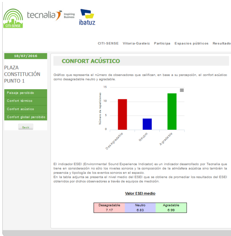
Figure 30: Visualization of Acoustic comfort results. It shows the number of users that evaluate the acoustic conditions as pleasant or unpleasant (or neutral). The table below shows the mean ESEI value in each group of evaluations.
