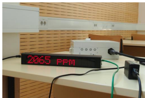
Figure 1: The CO 2 -sensor unit built by the students
